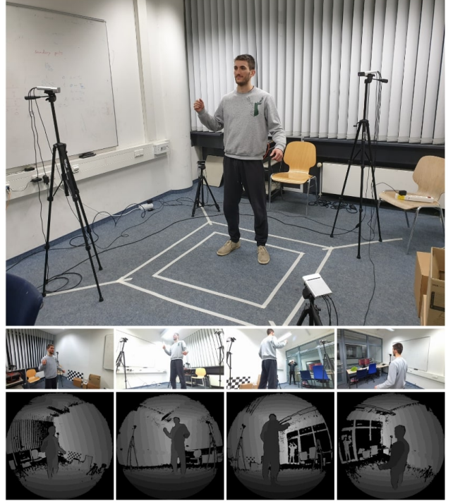
Figure 12: We capture non-rigid motion using 4 Kinect Azure sensors, which are pre-calibrated and hardware-synced to guarantee spatial and temporal coherence of depth captures. We capture depth images at resolution of 1024 \times 1024 , using the highest available frame-rate of 15 FPS.
